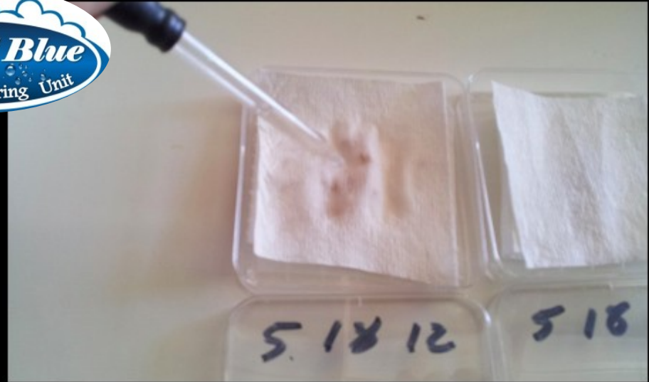
Apply enough water in equal amounts to each sample container to assure complete moistening of all test material
